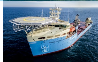
DeepOcean Maersk Connector power cable installation vessel
